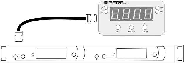
Illustration 3: Connecting PM-1 to an IEM TX(BNC)
