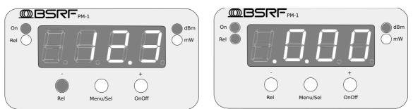
Illustration 4: While displaying power as dB press 1 sec Rel to switch to relative mode
