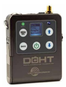
The DCHT/E01 transmitter is designed for use in film and television production to provide a wireless link from a bag or cart system to cameras and recorders. The transmitter will accept mic or line level analog signals or AES digital signals from a mixer and transmit the signals to the receiver in a pure digital format. The digital architecture is a third generation design with specially developed, high efficiency digital circuitry for extended operating time on two AA batteries.
