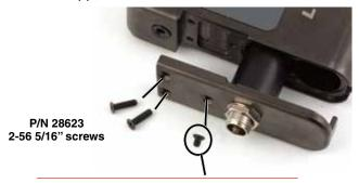
CAUTION: Use only the shorter screw P/N 28615 2-56 1/8" in the hole near the connector. The longer screws may damage a circuit board component.
