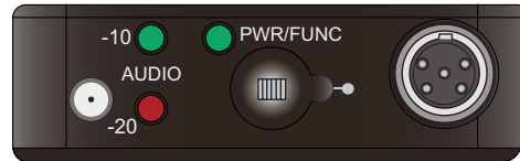
The top panel provides the antenna port, audio level LEDs, programmable switch and input jack.
