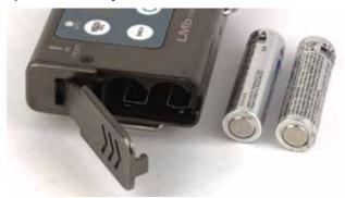
Spring contacts inside the compartment and nickel plated contacts on the door keep the batteries from rattling and provide reliable electrical contacts. The unit is protected from reverse battery polarity electrically, and by the insulated contact plate in the battery door.
