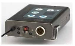
The servo bias input accepts mic or line level signals with a wide range of gain adjustment in 1 dB steps. Accurate LED indications on the top panel and a bar graph indicator on the LCD allow precise gain adjustments to achieve the maximum signal to noise ratio and minimum distortion. The limiter in the input preamp can cleanly handle signal peaks over 30 dB above full modulation, allowing the input gain to be set high enough to achieve the maximum signal to noise ratio.
