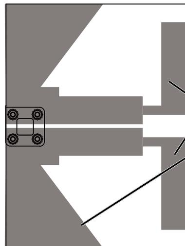
The antenna is constructed on a fiberglass printed circuit board for a slim profile and rugged structure.
