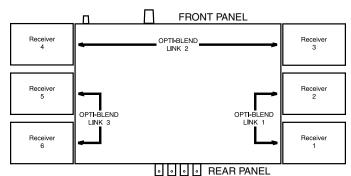
Ratio diversity employs a panning action that blends the RF signals from the two receivers over a fairly wide range of levels to eliminate dropouts before they occur. The process is called OptiBlend<sup>TM</sup> as indicated on the
