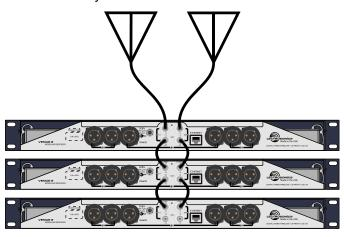
The built-in multi-coupler includes "loop through" outputs for stacking multiple Venue receivers.
