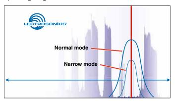
IP3 is used as a measure of a receiver's ability to reject strong RF signals near the operating frequency of a wireless system. When two signals that can generate IMD3 (third order IM) are even a few MHz away from the carrier, the iQ filter in the narrow mode suppresses them significantly. The already excellent IP3 performance of the receiver with the iQ filter in the normal mode is further improved when the filter switches to the narrow mode.
