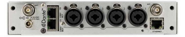
The M2T/E01 half-rack transmitter features transmission power of up to 50 mW for extended operating range. Locking XLR/TRS Combo connectors facilitate up to four channels of analog audio sources to be applied to the transmitter. A large, high resolution, backlit LCD and large membrane switches provide an intuitive interface.
