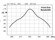
tive as most fixed frequency designs, with the overload performance of the best front-ends available. The result is extended operating range in even the most congested RF environments.
