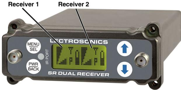
The control panel is a rugged, dust and water resistant design with membrane switches for the control interface. A backlit, graphics-type LCD is used to set up and monitor the receiver. Navigation through the menus is straightforward with text prompts for value and mode selections. In the ratio diversity mode, the Main Window displays audio levels, transmitter battery status, pilot tone status and RF level activity for both receivers, with a single audio channel display.
