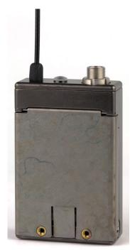
The battery cover is made of stainless steel for durability, and to preserve the thin wall thickness needed for a miniature design. The cover is hinged to the housing to simplify handling during battery changes.
